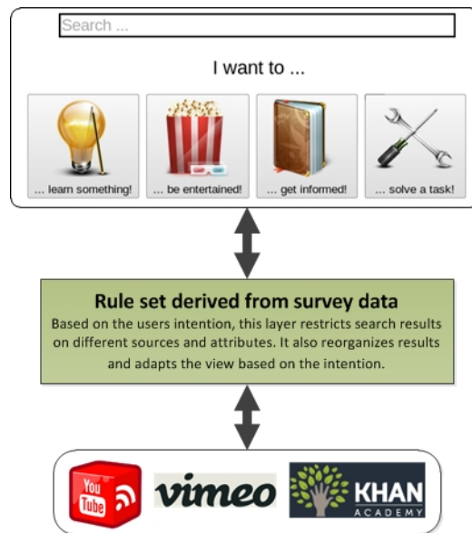
Figure 18: Block diagram of the prototype for an adaptive video retrieval system.
